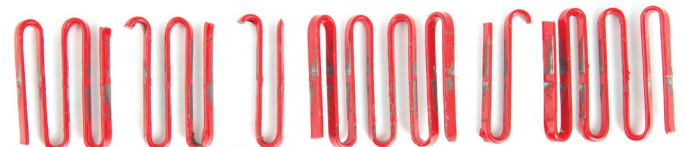
Dodge grid element after 70,000 cycles
