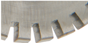
After 400,000 test cycles, Falk Steelflex hub shows no wear with smooth, machined surfaces.
