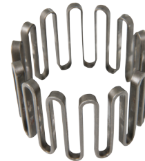
Falk grid element after 400,000 cycles
