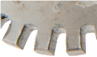
Competitive hub shows pitting on teeth and burrs on tooth edges from broken grid element.
