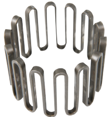
Falk Steelflex after 400,000 cycles
