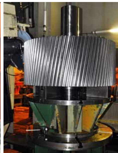
MR re-cut low speed gear at finish grind.
