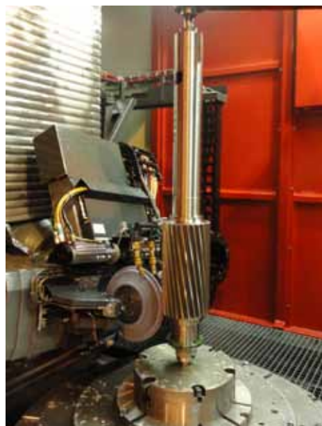
New main pinion at finish grind.
