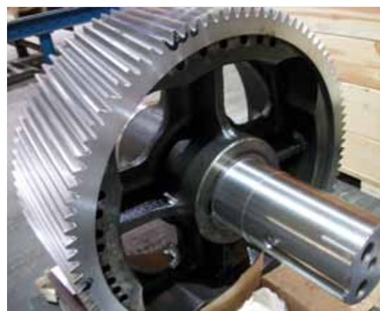
MR re-cut low speed gear at shipping.
