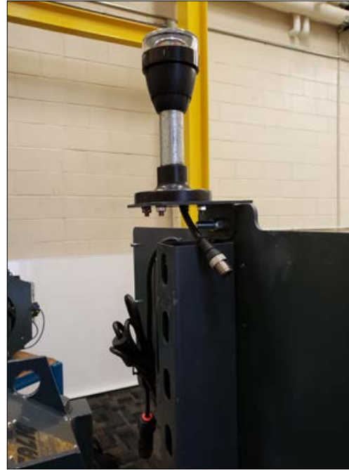
Figure 19 – Assembled view of Edge Device and Andon Light
