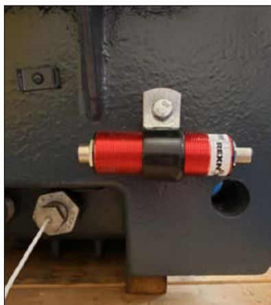
Figure 6 – Converter Installed on a V-Class Drive
