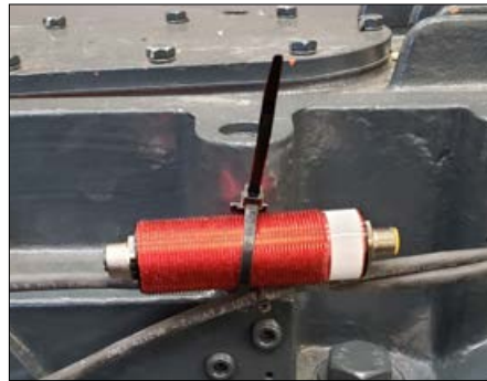
Figure 10 – Converter secured with cable mount
