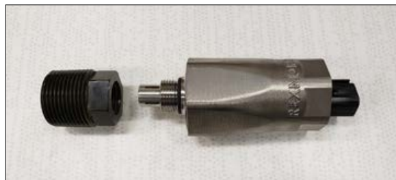
Figure 11 – Oil quality sensor components
