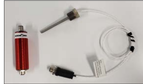
Figure 5 – Oil Sump Temperature Components
