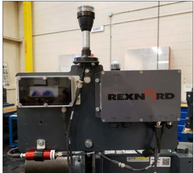
Figure 17 – Assembled view of Edge Device and Andon Light
